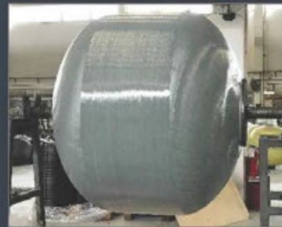
computer controlled filament winding
